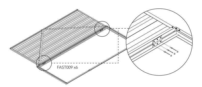
Lay the LEFT SIDE PANEL face up and lay the DOOR PANEL down in the open position on top as shown. Using three rivets per hinge, FAST009, secure the door to the frame. NOTE: Run the 3mm drill bit through the punched holes in the jamb before riveting the hinge on.
