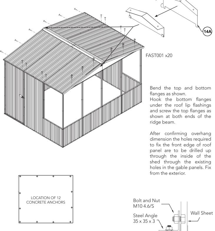
Each anchor consists of one nut, bolt, M10 dynabolt and steel angle. Drill a 10mm hole into the wall sheet. Drill a 10mm hole into the concrete.
