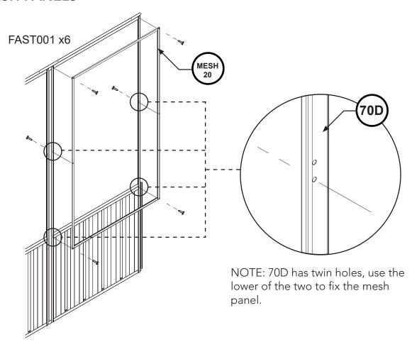
The mesh panels are fixed to the interior of the wall panels.
