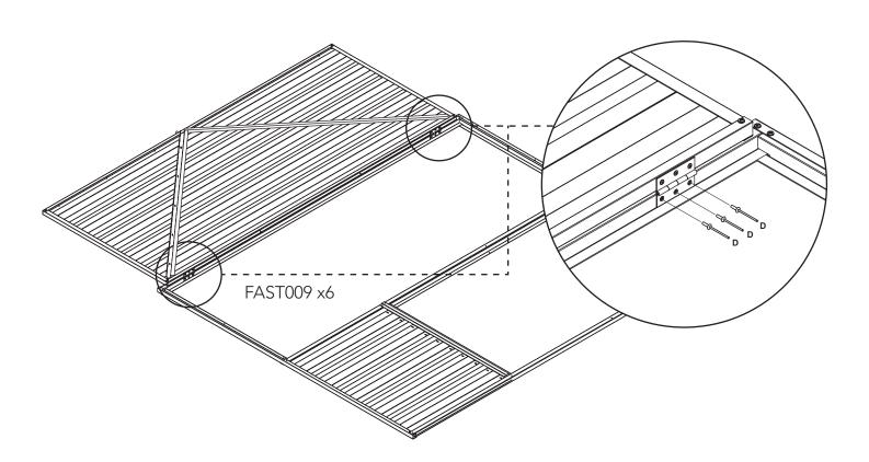
Lay the LEFT SIDE PANEL face up and lay the DOOR PANEL down in the open position on top as shown. Using three rivets per hinge, FAST009, secure the door to the frame. NOTE: Run the 3mm drill bit through the punched holes in the jamb before riveting the hinge on.
