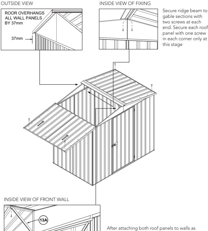
gable sections with two screws at each end. Secure each roof panel with one screw in each corner only at this stage
