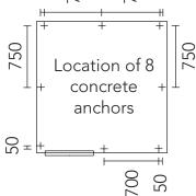
Each anchor consists of one nut, bolt, M10 dynabolt and steel angle. Drill a 10mm hole into the wall sheet.
