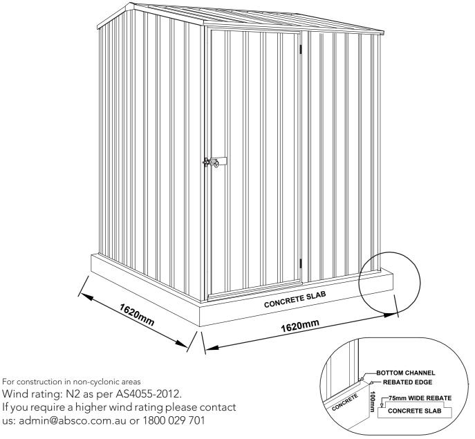
NOTE: This shed can be upgraded to wind rating: C1 as per AS4055-2012 with the additional purchase of a Cyclone Kit.
