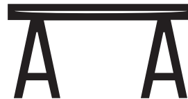
Raised work surface. EG Sawhorses and timbers
