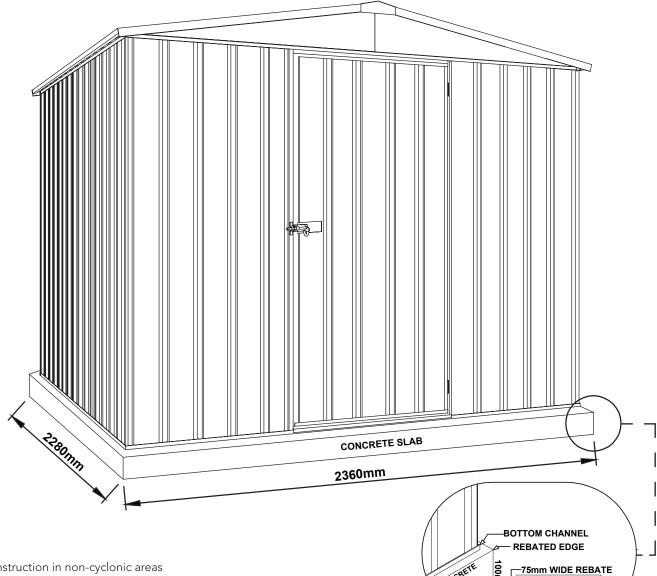
For construction in non-cyclonic areas Wind rating: N2 as per AS4055-2021. If you require a higher wind rating please contact us: admin@absco.com.au or 1800 029 701
