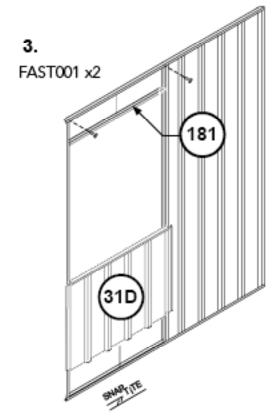
Notch out both bottom corners as shown using tinsnips.
