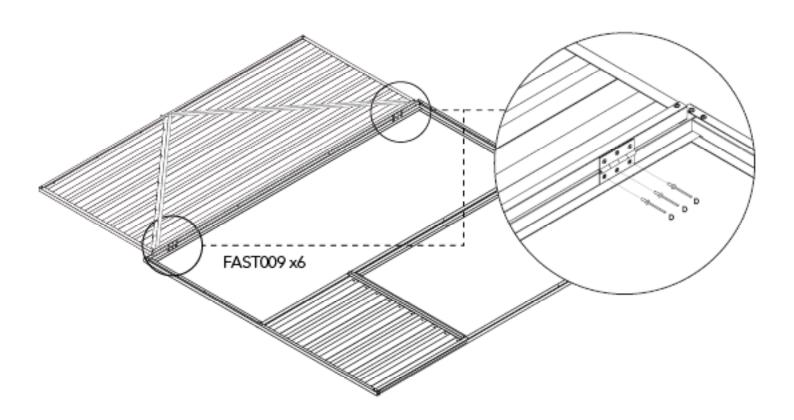
Lay the LEFT SIDE PANEL face up and lay the DOOR PANEL down in the open position on top as shown. Using three rivets per hinge, FAST009, secure the door to the frame.
