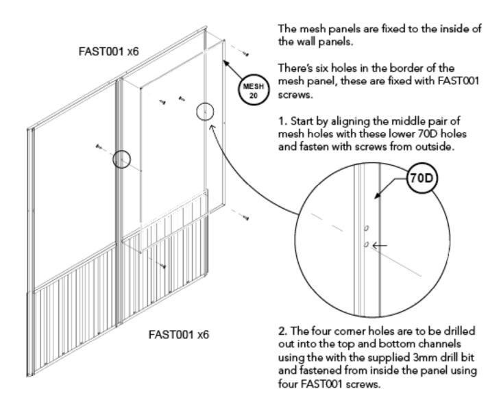
WARNING: It is recommended that new galvanised mesh should be weathered for two (2) months or scrubbed with a mild acidic solution, such as vinegar, then rinsed with water before being used in bird housing applications.
