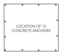
Each anchor consists of one nut, bolt, M10 dynabolt and steel angle.
