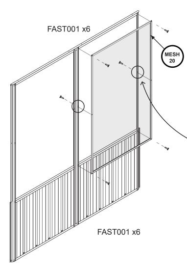
**NOTE:** If the mesh panel is not sitting flush enough for your liking you may drill more 3mm holes and fasten with additional FAST001. The mesh panels are fixed to the **inside** of the wall panels.
