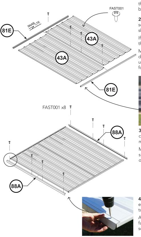
**1.** Overlap specified sheets as shown. Make sure ends are flush.
