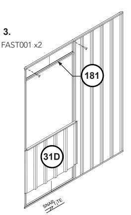
Notch out both bottom corners as shown using tinsnips.
