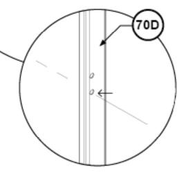
The four corner holes are to be drilled out into the top and bottom channels using the with the supplied 3mm drill bit and fastened from inside the panel using four FAST001 screws.
