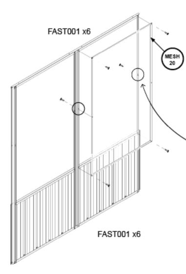
NOTE: If the mesh panel is not sitting flush enough for your liking you may drill more 3mm holes and fasten with additional FAST001. The mesh panels are fixed to the inside of the wall panels.
